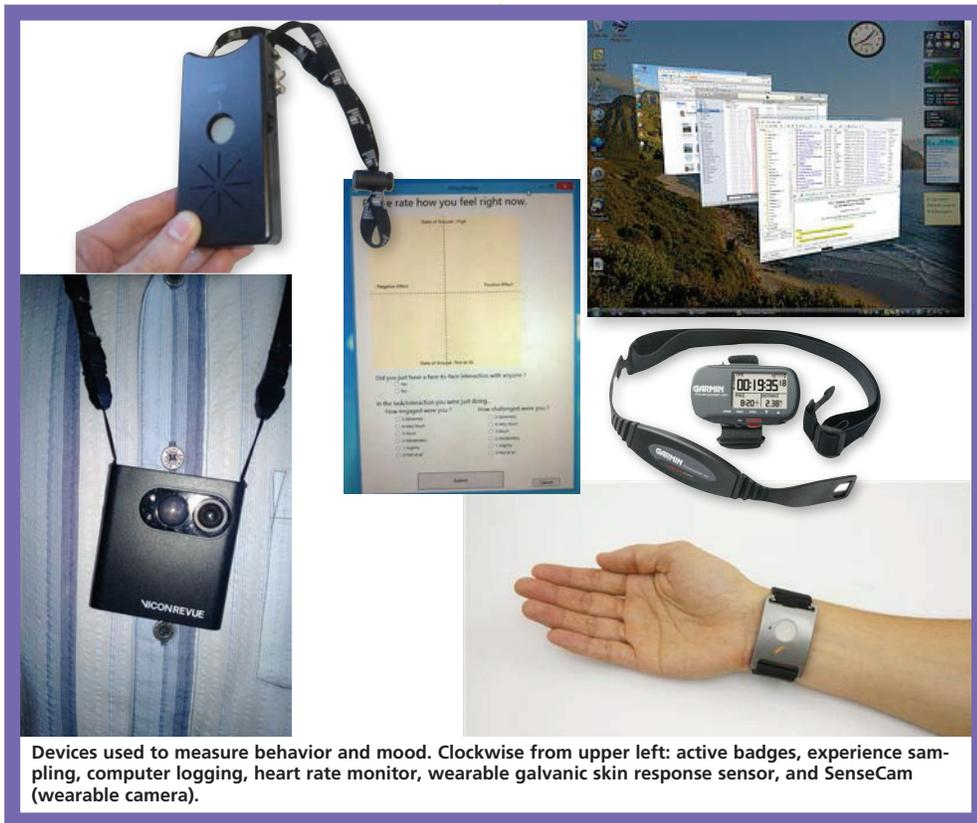
Devices used to measure behavior and mood. Clockwise from upper left: active badges, experience sampling, computer logging, heart rate monitor, wearable galvanic skin response sensor, and SenseCam (wearable camera).
