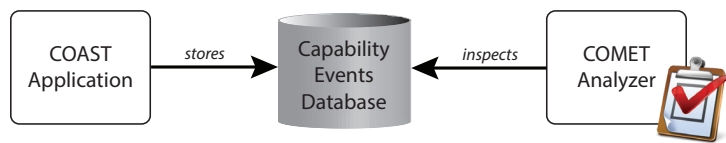
Figure 1: COAST applications capture capability events and store them into a database. COMET performs different types of analyses using the collected data.
